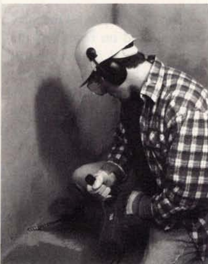
The new Kango 750 combination hammer with a multi-positional soft grip handle
